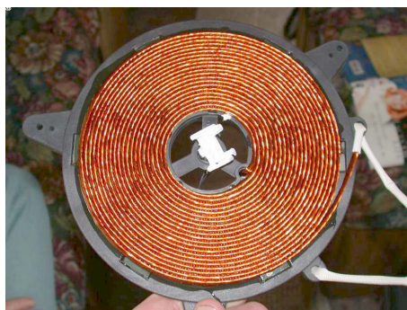
(a) Basic shape of the contactless power transfer coils.
