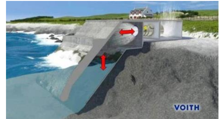
Oscillating wave surge converter / oscillating water column (water to air flow) Source: aquaret.com
