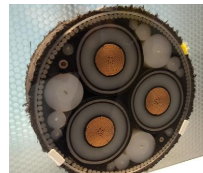
150 kV, 3-phase submarine cable
